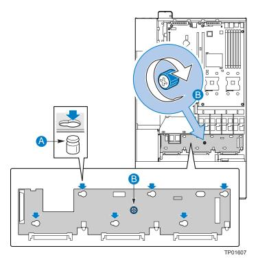
Figure 48. Installing a SATA or SCSI Backplane into the Chassis
